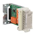
Relay discrete output module, Modicon TSX Micro, 8 outputs, 3.5W, overvoltage protection by zener diode, CONN
