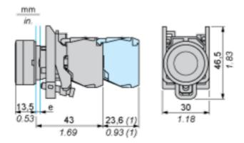
$\boldsymbol{e}$  : clamping thickness: 1 to 6 mm / 0.04 to 0.24 in. (1) Additional row of contacts or double contact
