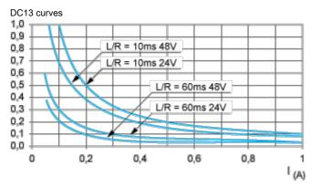
DC13 switching electromagnets,  $L/R \le 2 x$  (Ue x le) in ms, Ue: rated operational voltage, le: rated operational current (with a protective diode on the load, DC12 curves must be used with a coefficient of 0.9 applied to the number in millions of operating cycles)
