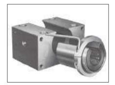
Place the mounting ring<sup>1)</sup> on as shown in the figure and use the adjusting screw to compress the radial linear bushing until it can be easily inserted into the housing bore by hand. The mounting ring hole must be about 0.5 mm larger than the outer diameter D of the radial linear bushing.
