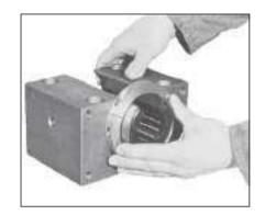
Once inserted, align the opening in the radial linear bushing with the opening in the housing and remove the mounting ring.
