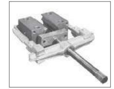
The preassembled radial linear bushing can also be pressed in with a puller. The pressure fitting must be on the ball bearings in the push rod (arrow). If this is not the case, an axial bearing must be placed on top of the push rod in order to prevent the torque that occurs from rotating the radial linear bushing in the housing.
