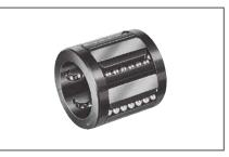
The radial linear bushings are high-precision linear bushings for moving extremely heavy loads. Radial ball redirection allows numerous rows of balls and extremely high load ratings.
