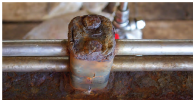
Crevice corrosion between the tube/tube trap interface.
