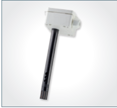
LK-SX Duct air quality sensor with up to 4x 0..10 V outputs for detection of CO 2 , VOC, humidity and temperature (page 250, 254-256)
