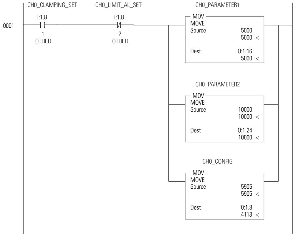
The rung below configures Channel 0 for 0 to 21 mA, sets the parameter option to “no action”, and holds the output in its last state on a fault condition. Note: 4113 decimal = 0001 0000 0001 0001 binary.
