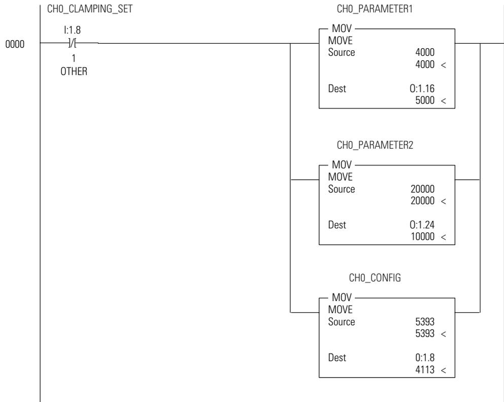
The rung below configures Channel 0 for 0 to 21 mA, sets the alarm limit range from 5000 to 10000, and holds the output in its last state on a fault condition.
