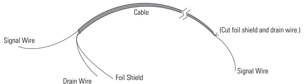
*Twist the drain wire and the foil shield together and connect to earth ground or to the chassis mounting screws.*
