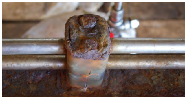
Crevice corrosion between the tube/tube trap interface.
