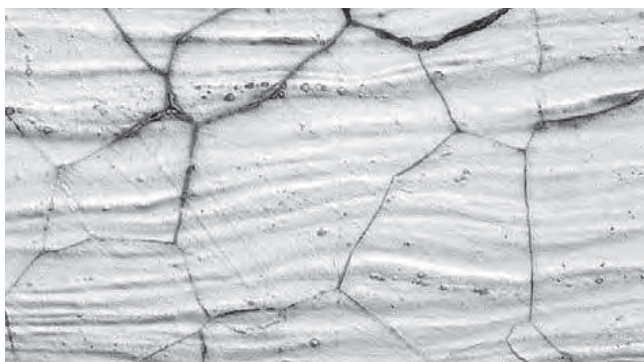
Intergranular Corrosion – HAZ Area – Stainless Steel Weld in Seawater Environment
