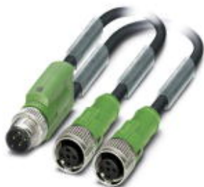
Sensor/actuator cable, 5-position, PUR halogen-free, black-gray RAL 7021, Plug straight M12 SPEEDCON, A-coded, on Socket straight M12 SPEEDCON, A-coded, PIN 2+4 bridged, cable length: 0.3 m
