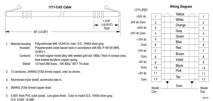
To connect the 1771-PS7 to non-IMC products, you must modify a 1771-CAS cable. Cut the cable as short as possible to minimize voltage losses. Double-up on +24V dc, +5V dc, +24V dc common, +5V dc common and 15V dc commons on each connector, as shown:
