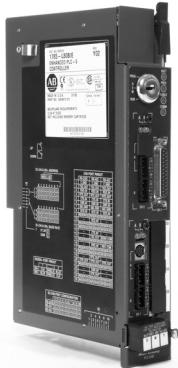
Every PLC-5 controller offers built-in, configurable ports for Data Highway Plus (DH+) or Remote I/O. A DH+ connection supports remote programming and information access, in addition to peer-to-peer communication between the PLC-5, other controllers, and devices. A Remote I/O connection supports real-time data exchange for I/O, operator interface, and other third-party devices.
