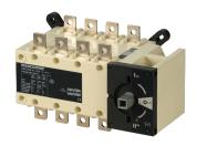
SIRCOVER products are manually operated transfer switches with positive break indication, for open-transition switching (I-0-II) available in 3 or 4 pole. They provide on-load transfer between two sources for any low voltage power circuit, as well as safety isolation by double breaking per pole. Other applications include source inversion (e.g. to change the direction of a motor) or grounding/earthing.
