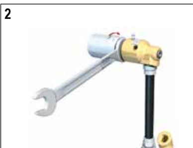
2 Install rotating union into machine.
