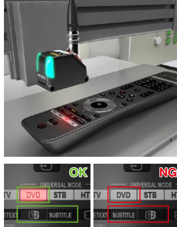
Remote control lighting check
