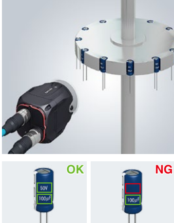
Capacitor marking presence
