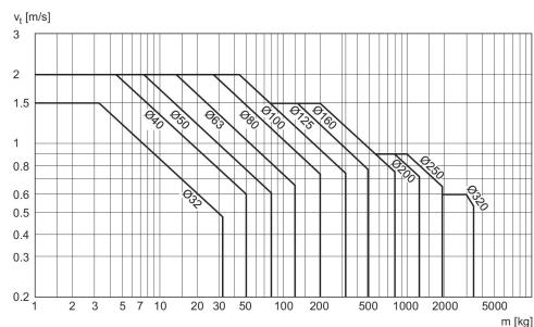
$v_t$  = Vitesse du piston [m/s] m = Masse amortissable [kg]
