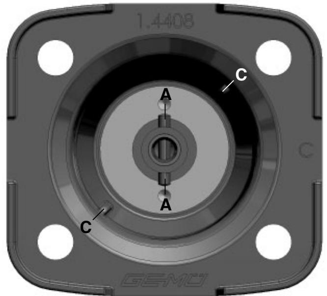
If the bonnet spindle is not in the correct position, it must be turned to the correct position. The position of **A** is offset by 45° to the position of **C**.
