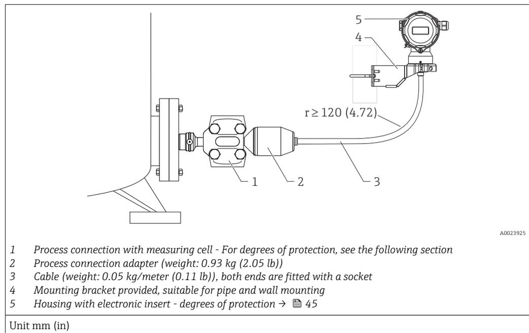
Degree of protection for the process connection and measuring cell with the use of
