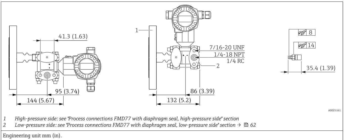
**Process connections FMD77 with diaphragm seal**
