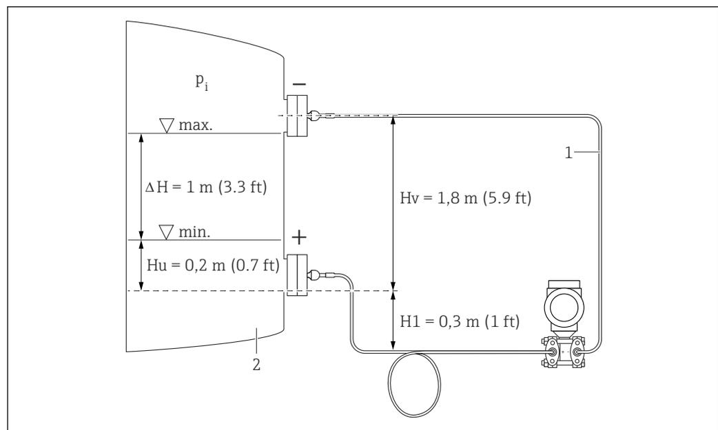
1 Capillary with silicone oil:  $\rho_{FI} = 0.96 \text{ kg (2.12 lb) dm}^3$
