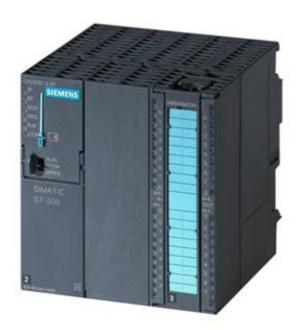
SIMATIC S7-300, CPU 313C-2DP COMPACT CPU WITH MPI, 16 DI/16 DO, 3 FAST COUNTERS (30 KHZ), INTEGRATED DP INTERFACE, INTEGRATED 24V DC POWER SUPPLY, 64 KBYTE WORKING MEMORY, FRONT CONNECTOR (1 X 40PIN) AND MICRO MEMORY CARD REQUIRED
