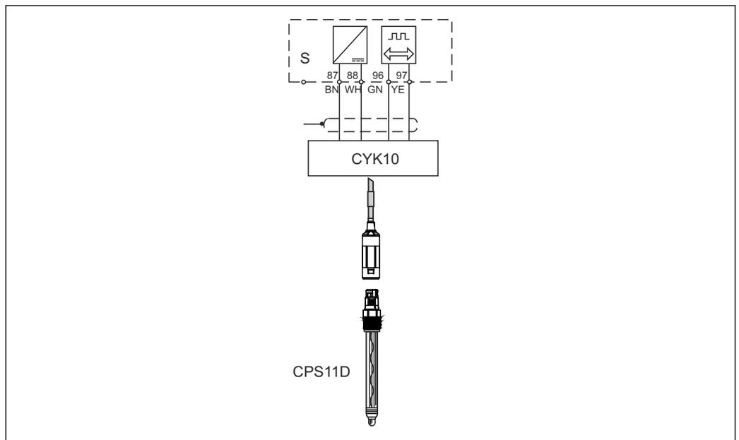
4 Connecting the digital sensor CPS11D with CYK10
