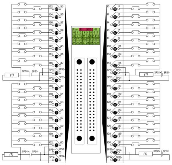
(1) fuse: fast blow fuse of 0.5 A for each 16-channel group power supply 24 VDC SPS sensor power supply
