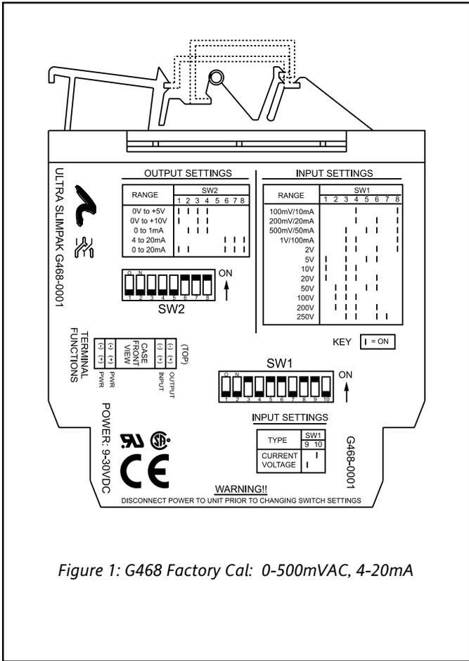
Figure 1: G468 Factory Cal: 0-500mVAC, 4-20mA
