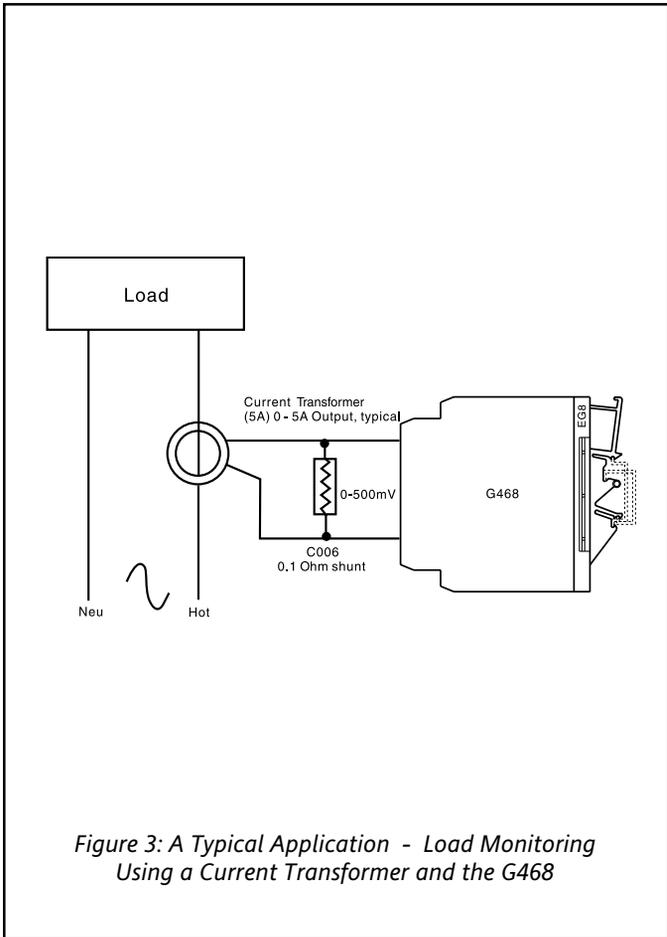
Figure 3: A Typical Application - Load Monitoring Using a Current Transformer and the G468
