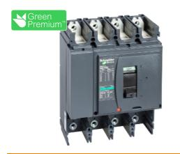
Circuit breaker basic frame, ComPact NSX400F, 36kA at 415VAC 50/60 Hz, 400A, without trip unit, 4 poles
