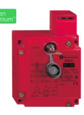
Safety switch, Telemecanique Safety switches XCS, metal XCSE, 2NC+1 NO, slow break, 2 entries tapped Pg 13, 24 V
