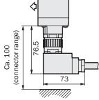
Angled cable socket M26 x 6 + FE with screw contacts
