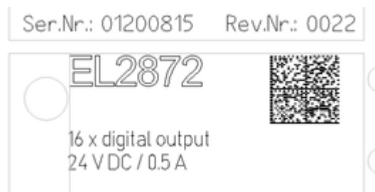
Fig. 1: EL2872 with revision 0022 and serial number 01200815
