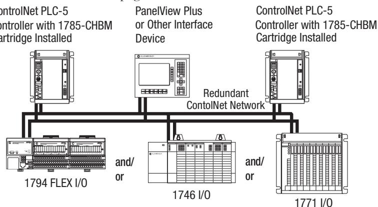
The PLC-5 Backup Communication Module, 1785-BCM, helps increase the fault tolerance of PLC-5 programmable controller systems controlling I/O on a remote I/O link by providing backup of the PLC-5 programmable controller.
