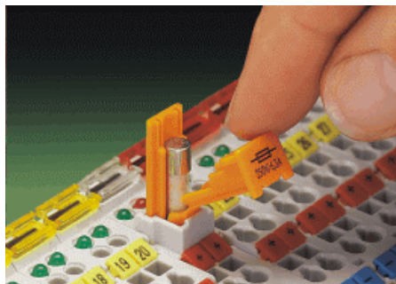
Fig. 2-16: Opening the fuse carrier
