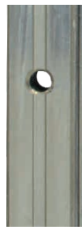
Rail (unloaded) with CZS coating – after 99 hours of salt spray test (according to DIN EN ISO 9227)
