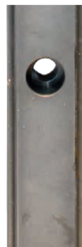
Rail (unloaded) with CTS coating - after 22 hours of salt spray test (according to DIN EN ISO 9227)
