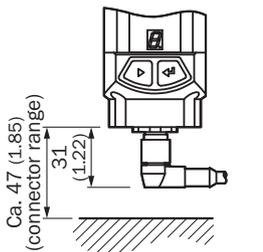
Cable socket M12 angled (only with AS-Interface: aligned)
