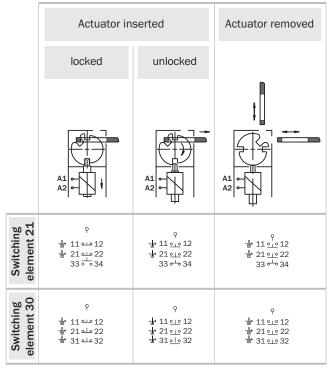
→ Positive action N/C locking monitoring contact
