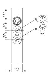
1) Output function, 2) Optical axis, 3) Light-on/dark-on, 4) Sensitivity
