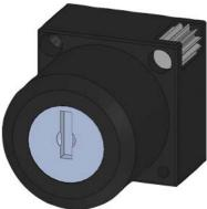
RONIS KEY-OPERATED SWITCH, 22MM, ROUND, PLASTIC, LOCK NO. SB30, WITH 2 KEYS, 2 SWITCH POSITIONS O-I, LATCHING, ACTUATING ANGLE 50 DEG.,12/14H, KEY REMOVAL POS. O, WITH HOLDER, POSSIBLE SPECIAL LOCKS: SB31, 421, 455 !!! Phased-out product !!! SIRIUS ACT 3SU1 is suc Preferred successor ty >>3SU1000-4BF01-0AA0 + 3SU1500-0AA10-0AA0<<
