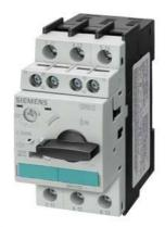
Circuit breaker size S0 for motor protection CLASS 10 A-release 11...16 A Shortcircuit release 208 A Screw terminal Standard switching capacity with transverse auxiliary switch 1 NO+1 NC !!! Phased-out product !!! Successor is SIRIUS 3RV2 Preferred successor type is >>3RV2021-4AA15<<
