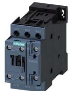
power contactor, AC-3e/AC-3, 25 A, 11 kW / 400 V, 3-pole, 24 V DC, auxiliary contacts: 1 NO + 1 NC, screw terminal, size: S0, upright mounting position
