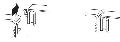
6. Push down and in at the same time to lock the adapter to the DIN rail. If the adapter does not lock in place, use a screwdriver or similar device to move the locking tab down while pressing the adapter flush onto the DIN rail, and release the locking tab to lock the adapter module in place.
